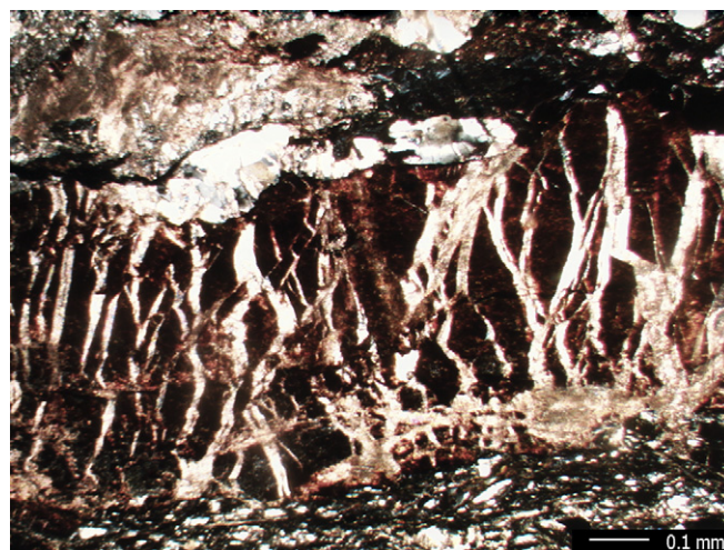
Fig. 2. Thin section image of sample KHS showing glassy or cryptocrystalline material associated with emplacement of microscopic carbonate (ankerite–calcite) veins.
